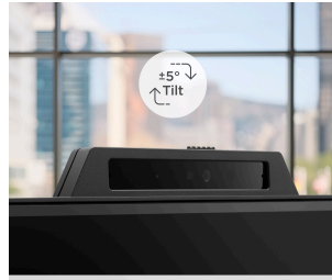
ADJUSTABLE BUILT-IN CAMERA With ±5 degree tilt and privacy shutter
