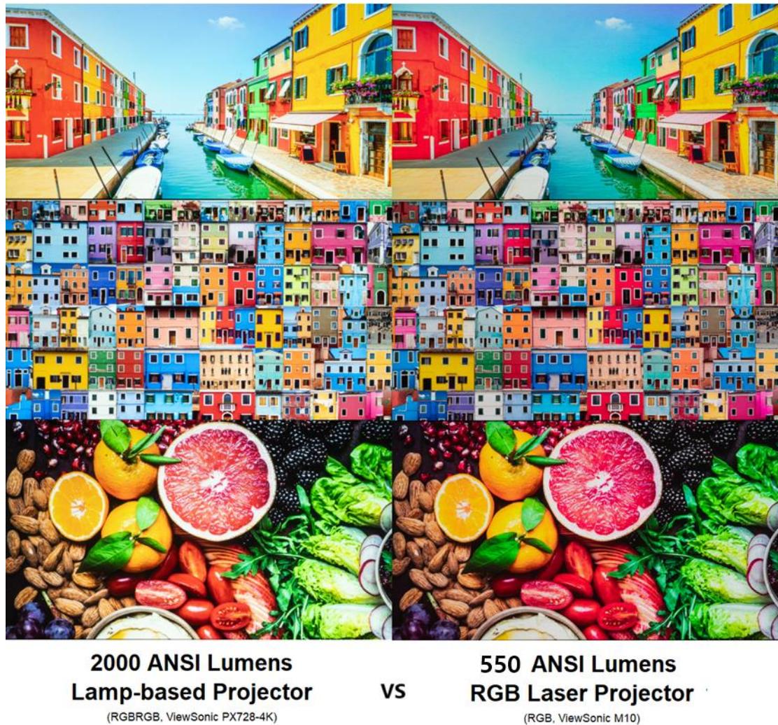
Figure 3. Sample image of a 2000 ANSI Lumens lamp-based projector (RGBRGB, ViewSonic PX728-4K) vs. a 550 ANSI Lumens RGB laser projector (RGB, ViewSonic M10)
